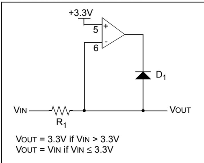
Because the clamping is performed by the op amp, there is no affect on the power supply. The impedance presented to the low voltage circuit is not improved by the op amp, it remains R<sub>1</sub> in addition to the source circuit impedance.
