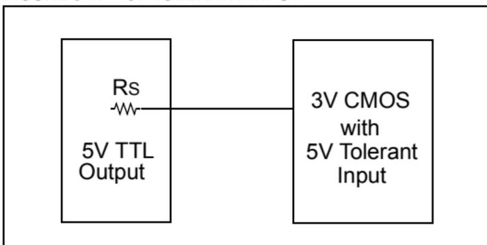
If the 3.3V CMOS input is not 5 volt tolerant, then there will be an issue because the maximum volt specification of the input will be exceeded.
