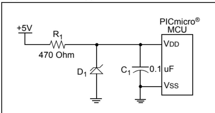
A simple, low-cost 3.3V regulator can be made out of a Zener diode and a resistor as shown in Figure 2-1. In many applications, this circuit can be a cost-effective alternative to using a LDO regulator. However, this regulator is more load sensitive than a LDO regulator. Additionally, it is less energy efficient, as power is always being dissipated in R<sub>1</sub> and D<sub>1</sub>.
