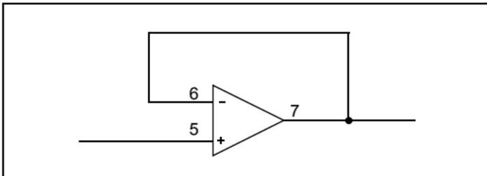
This circuit will output the same voltage that is applied to the input.
