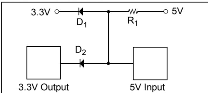
When output voltage specifications are determined, it is done assuming that the output is driving a load between the output and ground for the high output, and a load between 3.3V and the output for the low output. If the load for the high threshold is actually between the output and 3.3V, then the output voltage is actually much higher as the load resistor is the mechanism that is pulling the output up, instead of the output transistor.
